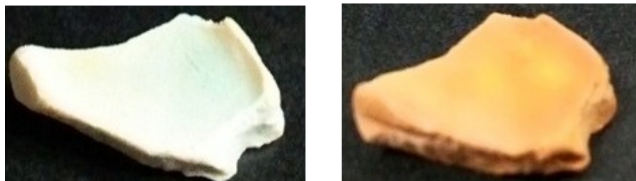
Figure 2.4.8 Photograph of the fluorenol polymer specimen before (left) and after (right) the hydrogen evolution.
