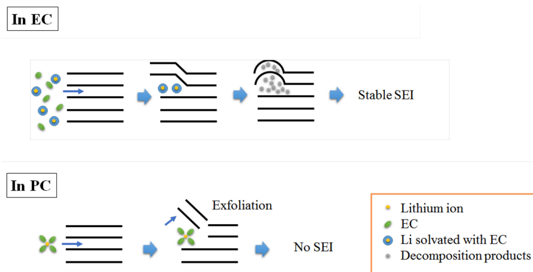
Figure 2.3.7 Schematic diagram of the mechanism of exfoliation of graphite layer and formation of SEI depending on solvent of PC and EC/DEC as electrolyte.
