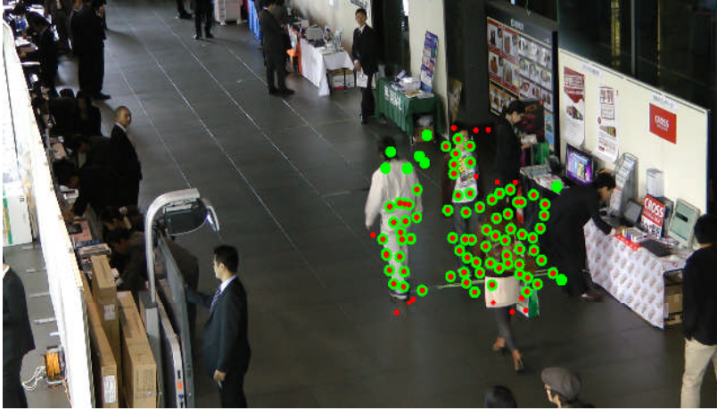
Figure 3.17: Keypoints of the MRF based method (red keypoints) and proposal (green keypoints).
