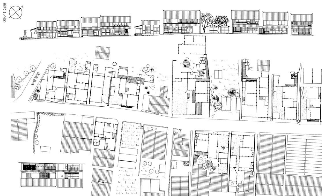
Fig.3.34 Fukugenzu plan of Gokoku area. Only the studied houses were included. The tōridoma of each house is represented in a dotted hatch. All the annex buildings in the rear were excluded. Source: Uchiko Town, 1978.
