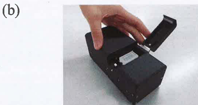
Fig. 1.4. (a) Optical arrangement of the whole WMR sensor using the Kretschmann configuration (After Ref. 18). (b) Photo showing a WMR sensor with four channels.
