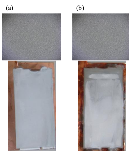
Fig. 3.27 Surface morphologies of Zn electrodes with 1.0 \text{ mmol dm}^{-3} \text{ In} at the capacity of 540 mAh at (a) -25^\circ \text{C} and (b) 50^\circ \text{C} .
