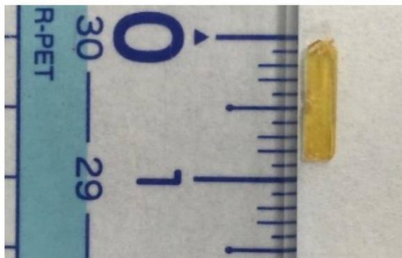
**Figure 2-1** Photograph of the  $[\text{Mn}(\text{H}_2\text{O})_2\text{Ni}(\text{CN})_4]\cdot 3\text{H}_2\text{O}$  single crystal as-synthesis
