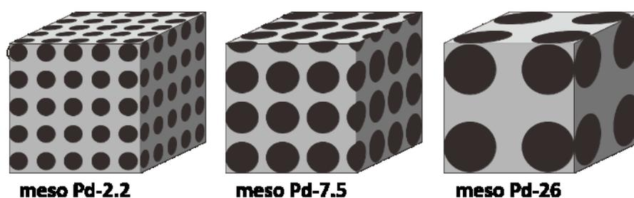
**Figure 2.28** Modeled pore arrangement and geometry of meso Pd-2.2, meso Pd-7.5, and meso Pd-26 for validating the calculation of the Pd surface area inside the films. To make these models, the pore sizes and the wall thicknesses were fixed to be 14 nm and 6 nm (for meso Pd-2.2), 25 nm and 6 nm (for meso Pd-7.5), 41 nm and 18 nm (for meso Pd-26), respectively.
