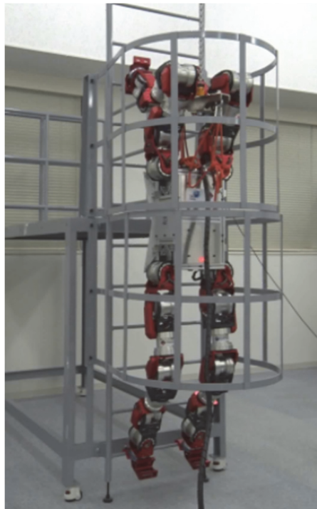
Fig. 2.9 WAREC-1 climbing a vertical ladder with safety cage.
