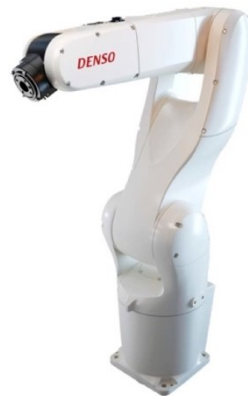
Fig. 5.7 6-DoF robot arm used in this study (VS-068) [5.5]
