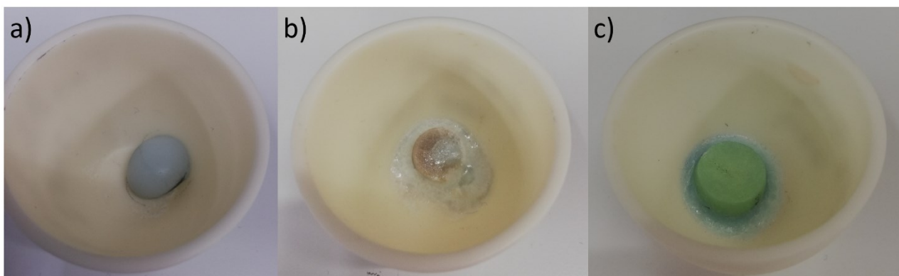
Fig. 6-7. Partially melted samples, a) Ca 3 Al 2 Si 3 O 12 at 1265 °C, b) CaSiO 3 at 1838 °C, and c) Ca 3 MgSi 2 O 8 at 1441 °C.
