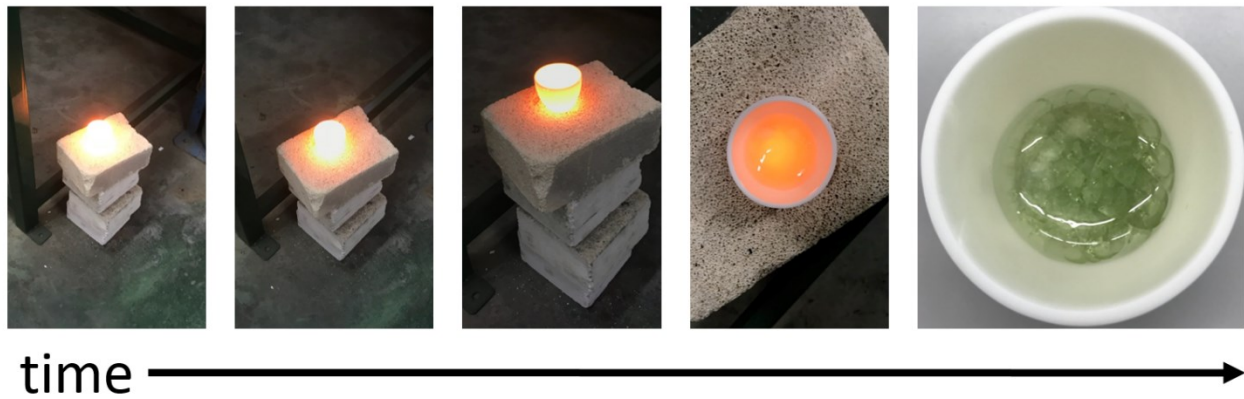
Fig. 6-12. Removal of liquid slag from the furnace for rapid solidification.
