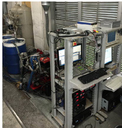
FIGURE 3.1: Diesel engine test bench
