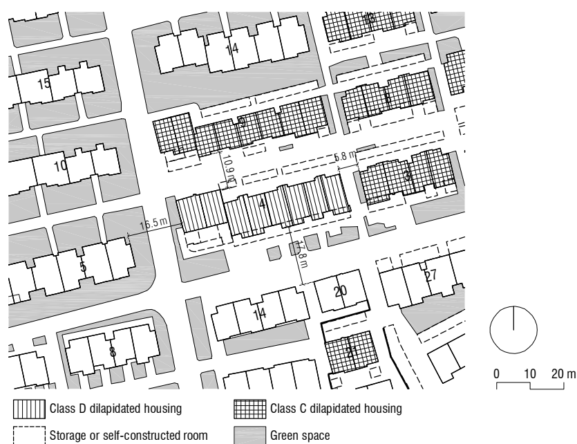
Figure 5-10 Distance between Building No. 4 and adjacent buildings
