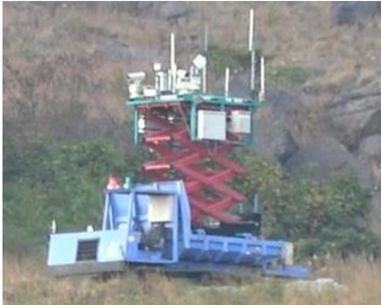
Fig. 1.7 Picture of environmental relay cars used for unmanned construction work ordered by Unzen Restoration Work Office, Ministry of Land, Infrastructure and Transport, and constructed by Asunaro Aoki Construction Co., Ltd.
