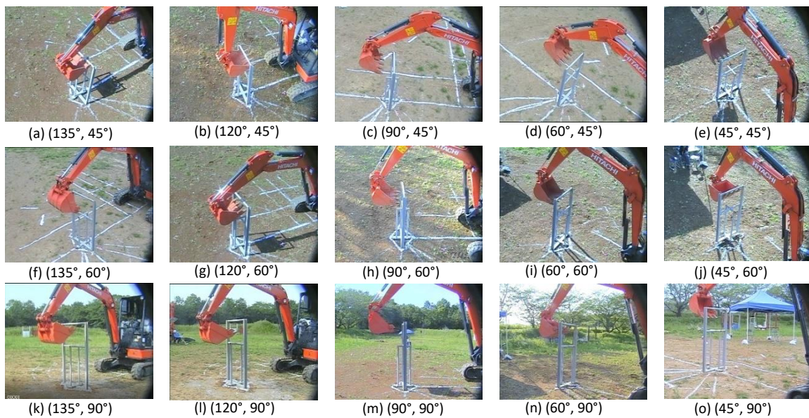
Fig. 3.17 External views under each condition, where (x^\circ, y^\circ) represents (pan angle, tilt angle)
