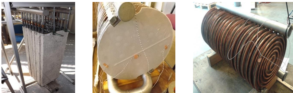
Fig. 2.5. Picture of a packed bed and heat exchanger (left) and the evaporator/condenser from the front (middle), and back (right) [10].
