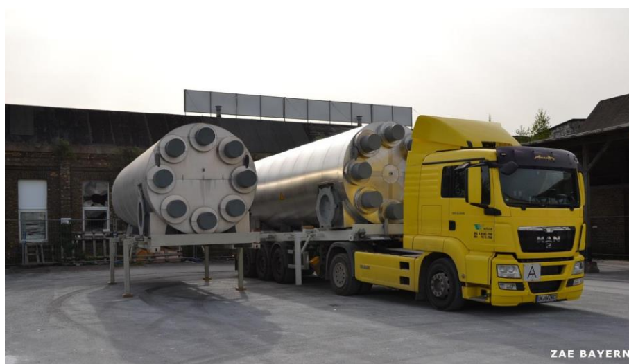
Fig. 2.14. Picture of mobile sorption reactor [23].
