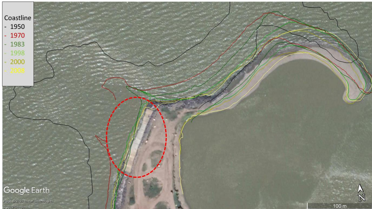
Figure 14. Over the years various approaches have been tried to protect the coastline of Tuktoyaktuk. One of the more successful protective measures have been using concrete slabs (red circled area). The relative effect can be seen with surrounding area to east, where changes have been more pronounced. Compiled from data provided by Hynes et al. 2014.
