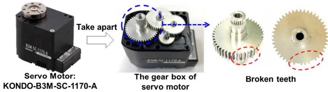
Figure 3.14. Gear teeth fractured by being subjected to unexpected loads by the user during walking.
