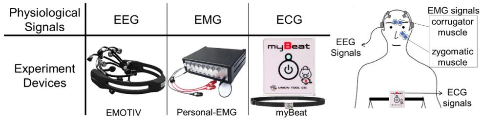
**Figure 4.7.** Three devices, EMOTIV, Personal EMG, and myBeat, used in the elicitation experiments.
