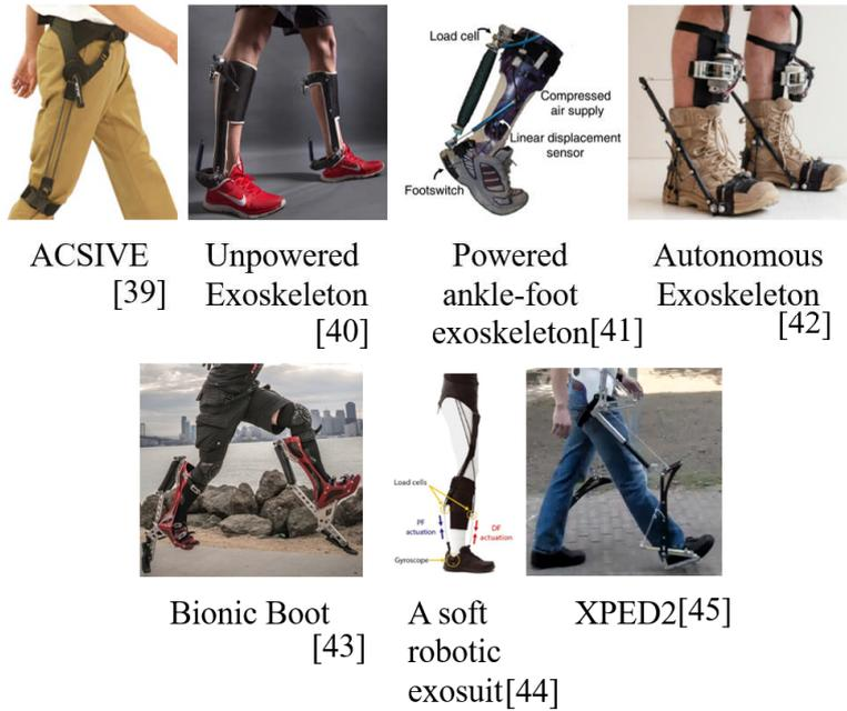
**Figure 2.2.** Wearable assistive devices of walking augmentation.
