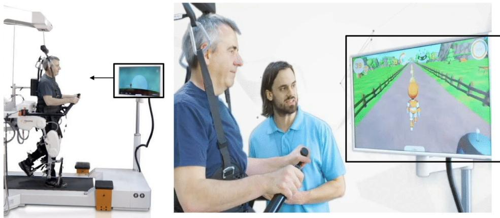
**Figure 2.3.** The device (Lokomat) used for rehabilitation by assisting three joint of lower limbs [120].
