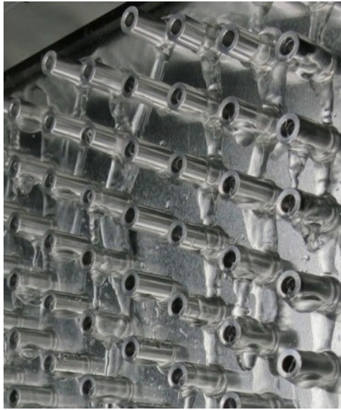
Fig. 3.1 Wetting phenomena, showing partial wetting, on the surface of a fin-tube substrate.
