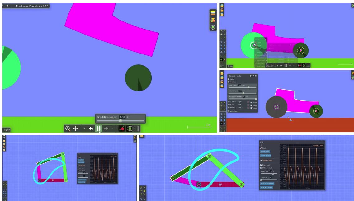
Figure 1.17: An interactive 2D physics simulation called Algodoo is an educational software that can be enjoyed like a game. It can also be used to simulate a mechanism such as a linkage mechanism to verify its operation.
