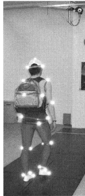
Fig. 2.3 Measuring motion and ground reaction force [36]
