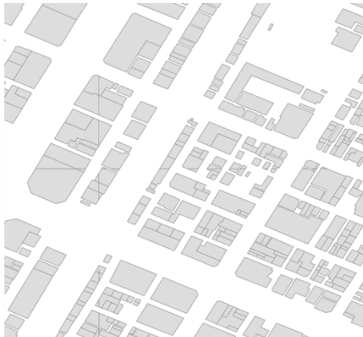
Fig.2-2-1 Polygons broken up by map boundaries (ex. Tokyo: 1996).
