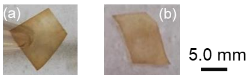
Figure 4.6 Optical images of NiP electroless deposition and Sn process: After (a) catalyzation and (b) electroless deposition
