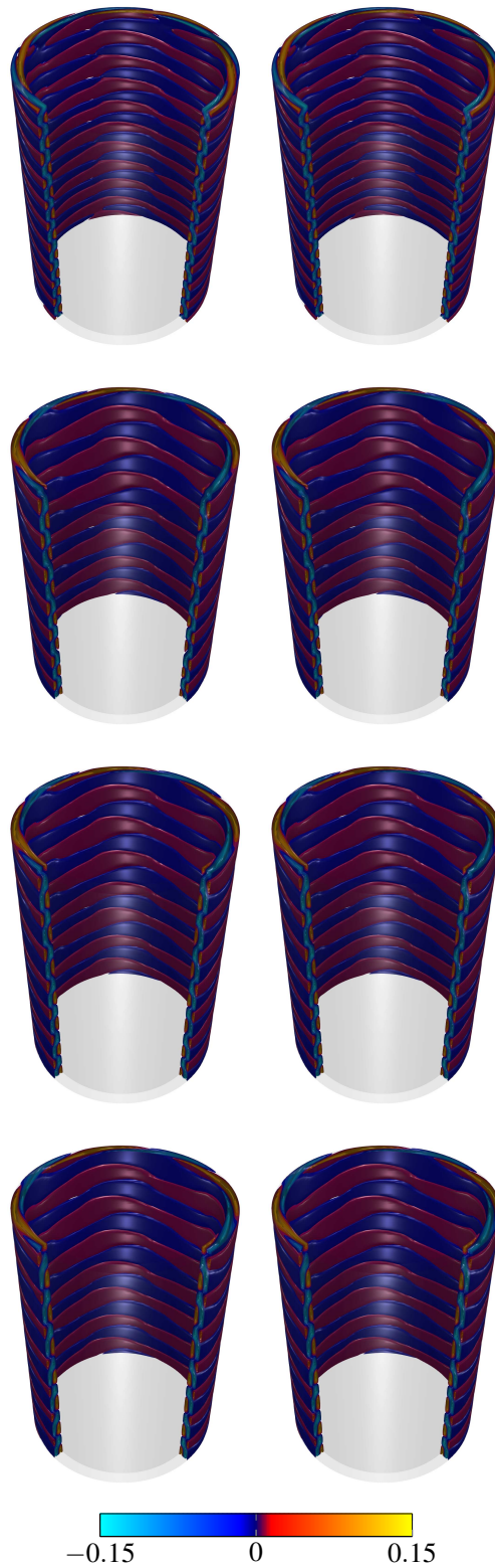
Figure 6.7: Flow development in Case 1. Isosurfaces of u_z / (U_i - \eta U_o) in the IRF ( left ) and NRF ( right ), with the full-domain representation of the flow field using the coarse mesh, at t = 10T, 30T, 50T and 70T (from top to bottom ). 16 isosurfaces are used in -0.15 \leq u_z / (U_i - \eta U_o) \leq 0.15 . This figure was also shown in [2]
