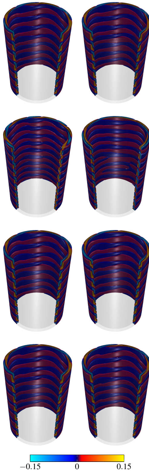
Figure 6.11: Isosurfaces of u_z / (U_i - \eta U_o) in Case 1 in the IRF ( left ) and NRF ( right ), with the quarter, one-third, half-domain and full-domain representations of the flow field (from top to bottom ), after the solutions become periodic. 16 isosurfaces are used in -0.15 \leq u_z / (U_i - \eta U_o) \leq 0.15 . This figure was also shown in [2]
