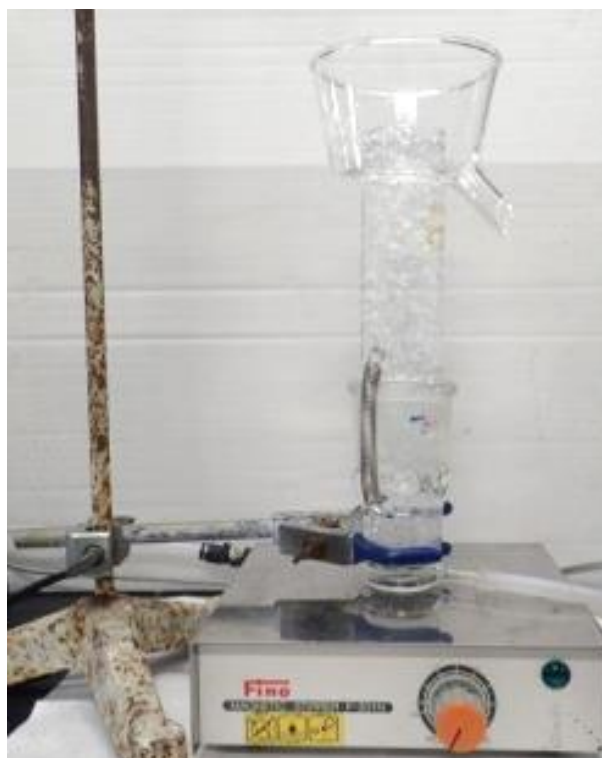
Fig. 3.3 The small column flotation apparatus.
