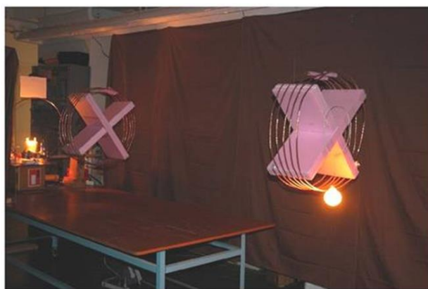
Figure 2.1 An experimental demonstration of wireless power transfer using magnetically coupled resonators (quoted from[7]).
