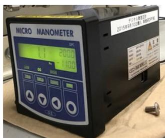
**Fig.2.40 Pressure sensor**
