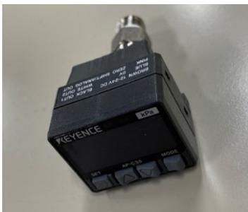
Fig.2.35 Pressure sensor
