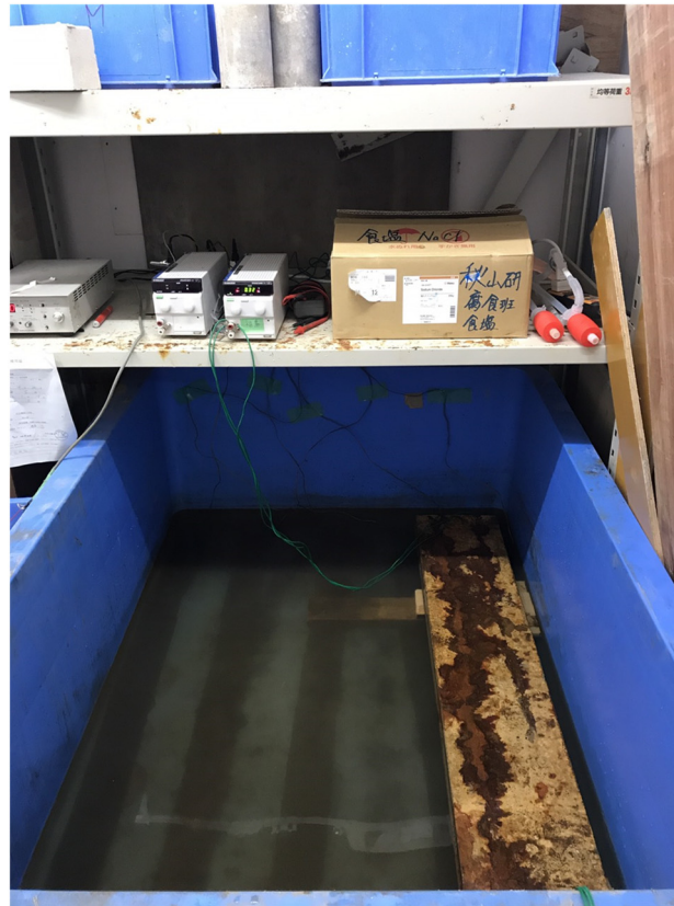
(b) Photograph of the experimental setup for the accelerated corrosion test on the RC slab specimen.
