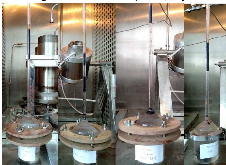
Figure 4. The imbibition process, Day 3.
