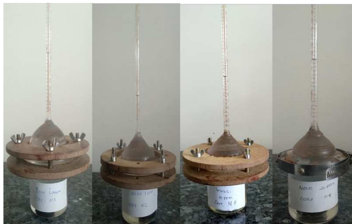
Figure 2. The imbibition process, Day 1.
