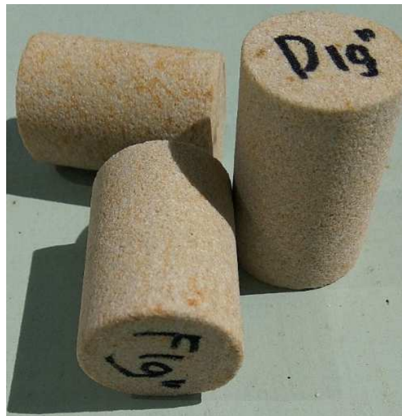
Figure 3.2. The Bentheimer SS core plugs.
