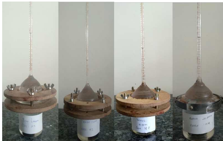
Figure 1. The imbibition process, Day 0.
