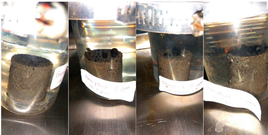
Figure 9. Core condition at sixth day of imbibition process
