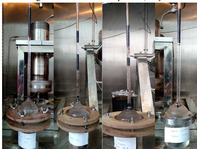
Figure 5. The imbibition process, Day 4.
