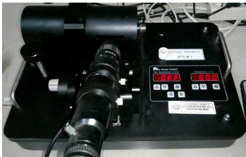
Figure 3.5. Spinning drop tensiometer instrument.
