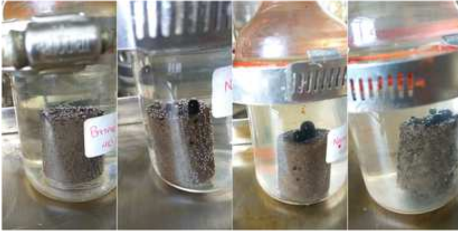
Figure 8. Core condition at first day of imbibition process
