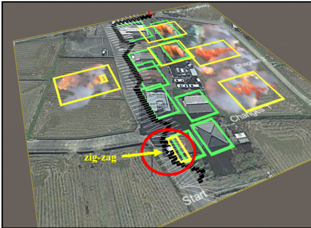
Fig. 3.7 Zig-zag Issues after Diagonal Node Expansion Algorithm
