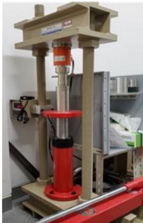
**Figure 3-12 Static compression device**
