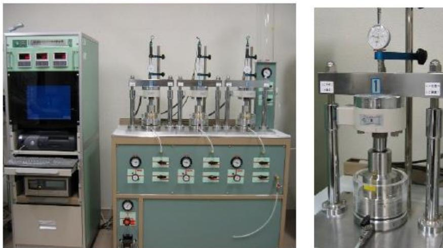
**Figure 1-17 Hydraulic conductivity for bentonite by compression apparatus (from Butsuda 2006)**
