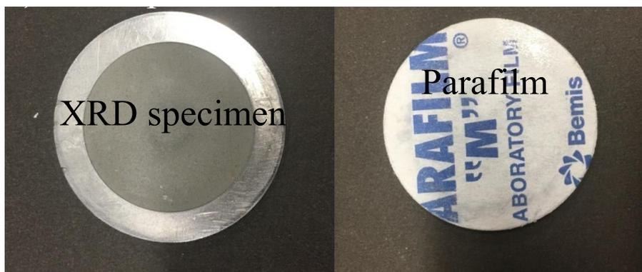
**Figure 10-4 2mm specimen for XRD tests and specimen sealed by parafilm**
