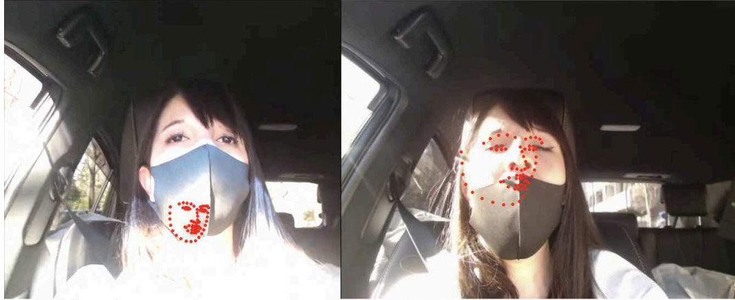
Figure 6.7: In Experiment 1.1, the method demonstrated poor performance in face detection, and in the few cases where it was able to recognize the face, it also struggled to identify landmarks.
