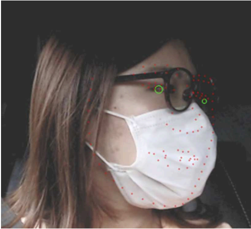
Figure 5.12: Example of miss-classification on Experiment 2.c with profile faces. The pupil tracker may fail when the driver has very thick eyeglasses frames.
